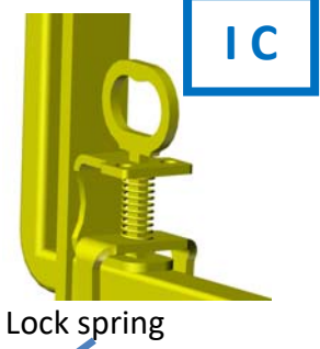
Bolt to fix the stability
