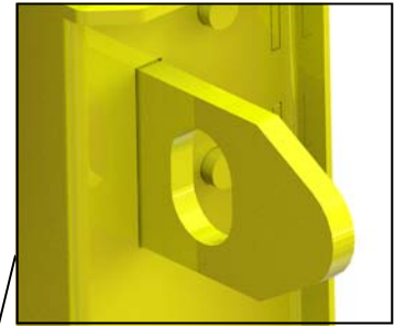
Ring to open and close panels
