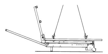
Step 3 Lift the folding scaffold ca. 2 m with the crane and secure the diagonals with the bolts (1 + 2). The folding scaffold is now ready for use.
