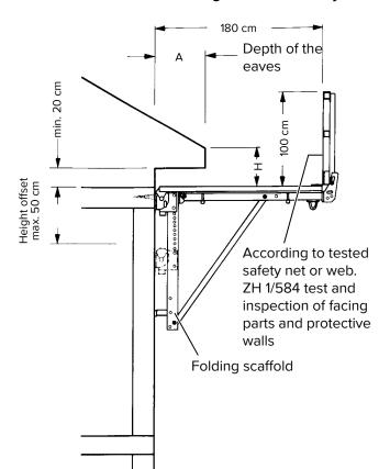
Diagram for the determination of the maximum height position of the facing dependent on the depth of the eaves.
