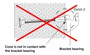
3. the cone anchoring is fixed to the reinforcement of the wall
