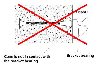
2. the anchor cone with the anchoring is mounted horizontally and vertically in a right angle to the form sheet
