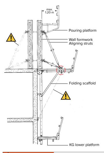
Detail: Mounting of the aligning struts (only possible in bracket axis)
