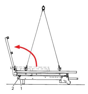
Step 2 Remove the bolts (1) for the shipping lock and the bolts (2) securing the diagonal tubing. Then remove the diagonal tube from the vertical strut of the platform of the folding scaffold.
