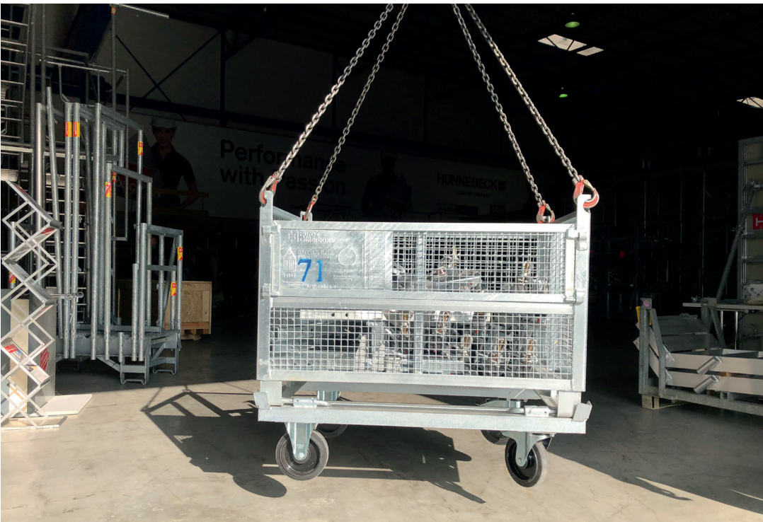
▶ The lattice box enables the storage of connectors, tie nuts, etc. It can also be attached to a trolley and moved by crane. The ease of handling saves considerable crane time – a distinct improvement for warehousing and logistics.
